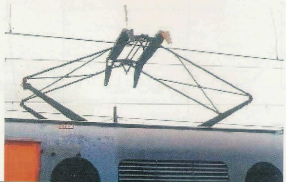
Figure 2: Problem: To model and redesign the overhead electricity collection system for a train pantograph to ensure contact is maintained throughout.
